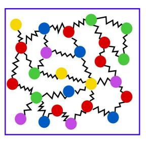
guide to the problem. When an amorphous structure is deformed, the response of the system is typically very jerky and intermittent. At sufficiently low temperatures, stress-strain curves display drops related to avalanches of motion.
