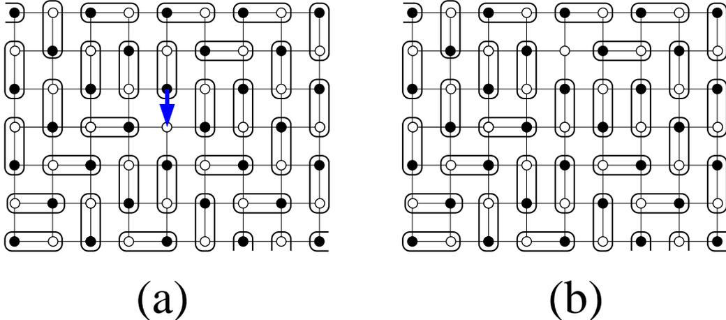
**Fig. 1:** An example of a dimer move on the square lattice. The dimer slides into the empty site (vacancy) of configuration (a), resulting in a new configuration (b) where the vacancy has jumped by two lattice spacings.
