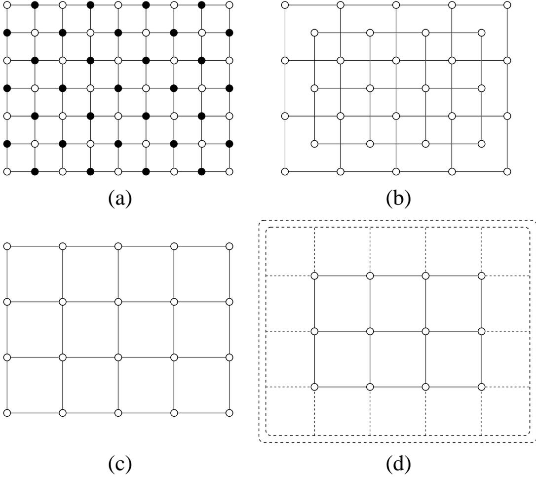
**Fig. 2:** A  $9 \times 7$  grid (a) is bicolored with one more white than black vertex. The set of white vertices is made of two intercalated grids of double mesh size (b) with respective sizes  $5 \times 4$  and  $4 \times 3$ . The first one (c) will be referred to as the odd white grid and the second one (d) as the even white grid. The latter is extended (dashed lines) so as to include an extra vertex (here represented by a double boundary) dual to the exterior face.
